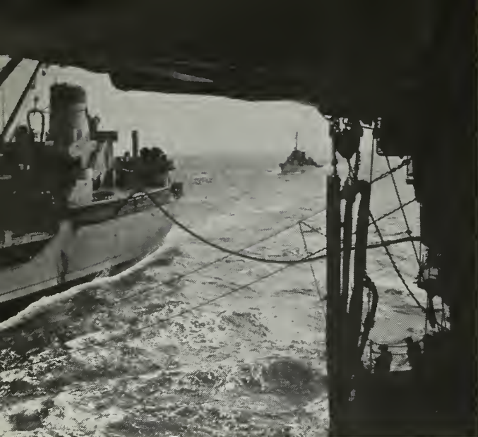
ON THE GO—Supplies and fuel are highlined to Seventh Fleet task force while underway in Pacific Ocean.
